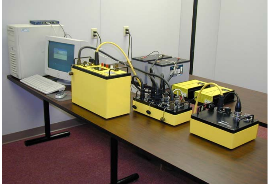
SuperSting Remote equipment set-up at the monitoring site.
