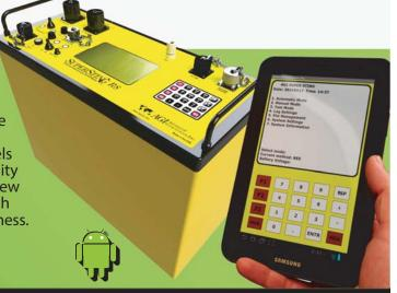
The instrument uses a built-in power transmitter and can be used for traditional vertical electrical sounding (VES), mise-a-la-masse measurements, or multi-electrode electrical tomography in 2D, 3D and 4D (time lapse). Other applications include borehole-to-borehole tomography, underwater measurements in rivers, lakes, dams and towed array investigations over water.
