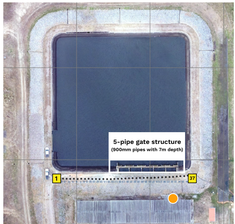
● The location where the leak was visible on the surface (10L/s)
