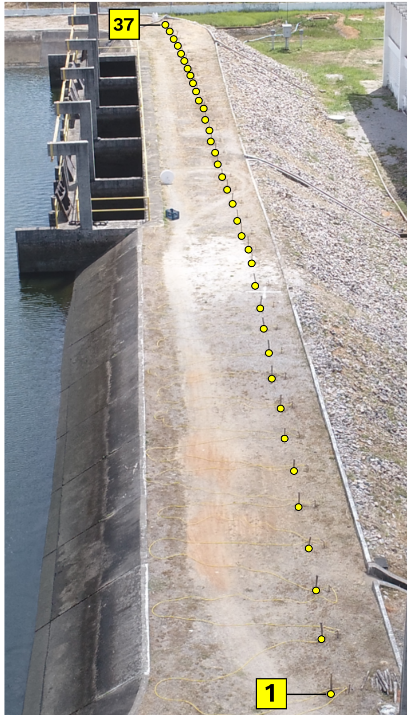
Pictured above: The placement of the 37 electrodes installed on the dam's crest. The space between each electrode was 2m.
