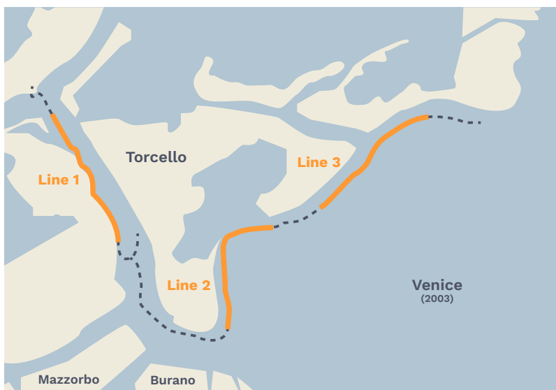
Figure 2 - The dashed lines were the GPS track of the boat. Resistivity data was collected along orange lines 1-3.
