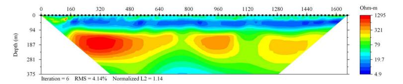
Example of Schlumberger, dipole-dipole and pole-dipole joint inversion using EarthImager 2D.
