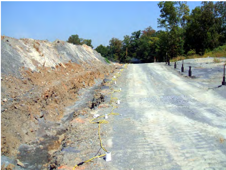
The non-polarizable electrodes (sensors) were buried along the survey profile
