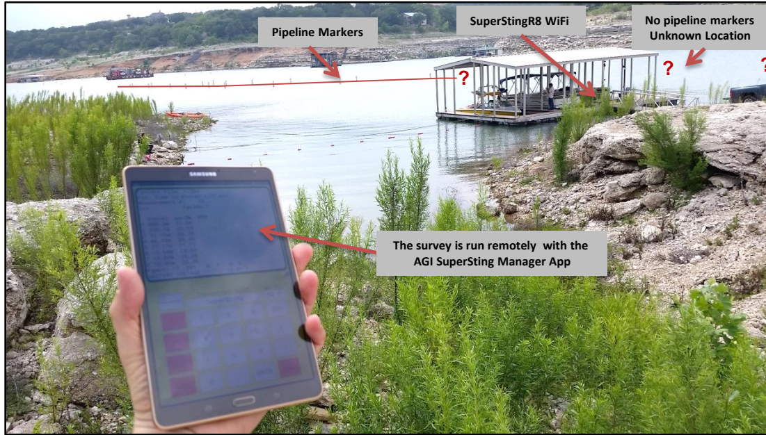
In the 2015 survey, full remote control with real time pseudo-section plotting was used to operate the instrument.
